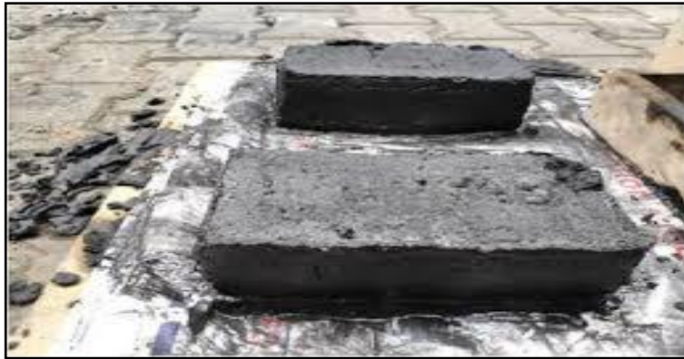
Utilization of sugar mill waste in the manufacturing of bricks
