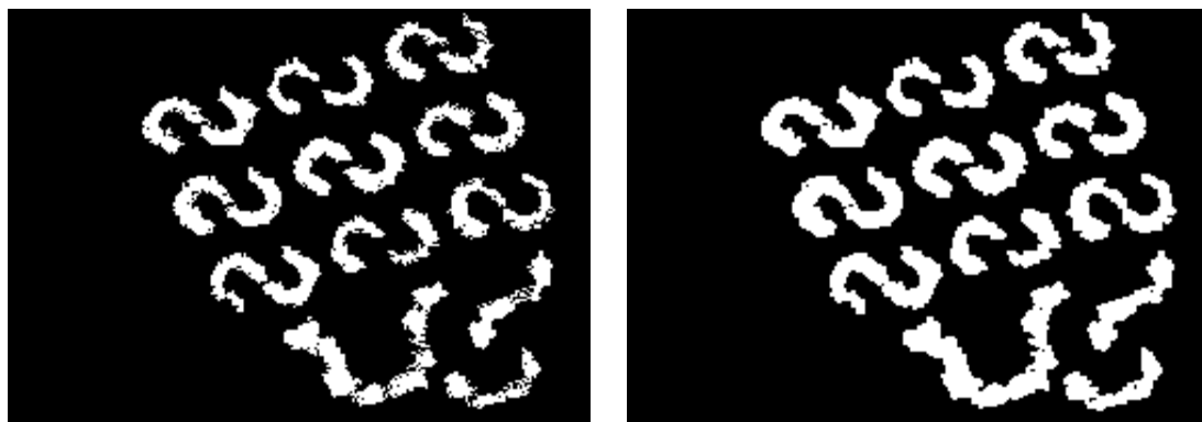
Figure 7. Segmented Building Regions Before (Left) and After (Right) Image Morphology for Scene-
