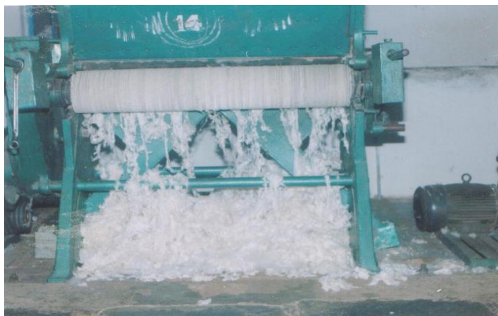
Figure 7. Photograph of a pilot model roller gin assembled with pollution-free RCF chromeless rollers
