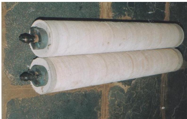
Figure 13. Rubbers having two layers of cotton fabric
