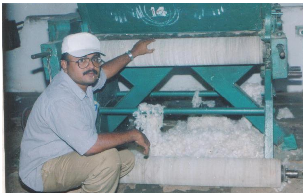
Figure 17. Newly developed eco-friendly, chrome-free RCF rollers assembled in existing DR ginning machine
