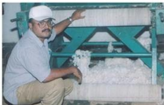
Figure-9: Green Design of Gin Rollers of Double Roller Cotton Ginning Machine
