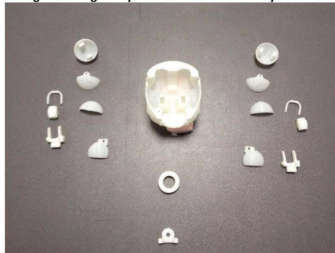
Figure 4. Head structure printed with creativity 3D minibot 3D printer
