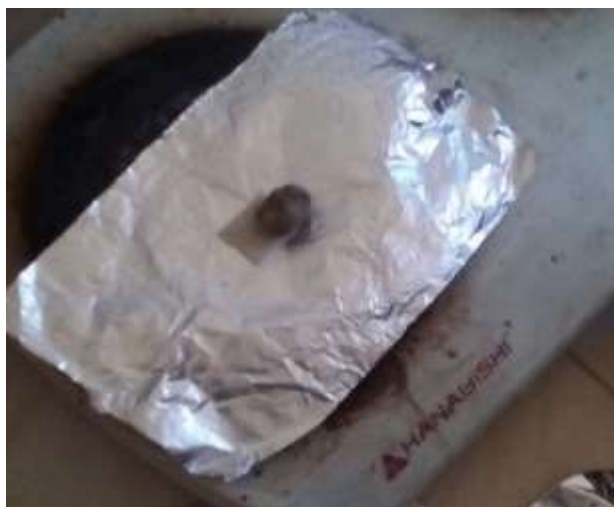
Figure 7. Setup of Improved Differential Scanning Calorimeter
