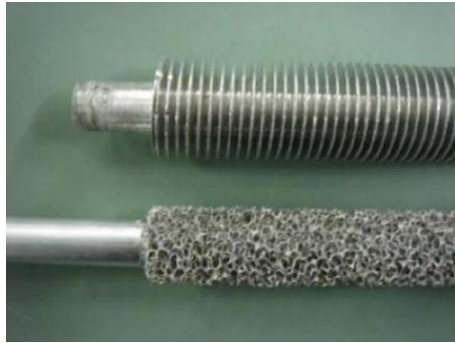
Figure 2. Helically finned tube and metal foam covered tube (T'Joen et al., 2010)
