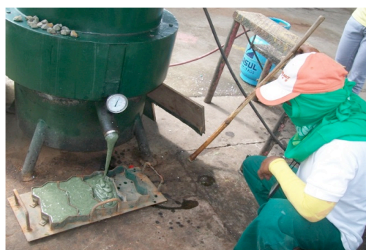
Figure 2a Molding of molten waste plastic by casting
